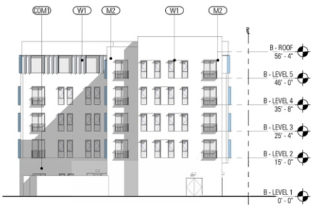
2 SOUTH ELEVATION - BLDG B A302 1/16" = 1'-0"
