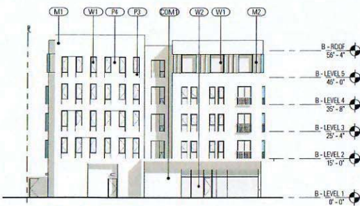
4 NORTH ELEVATION - BLDG B A302 1/16" = 1'-0"
