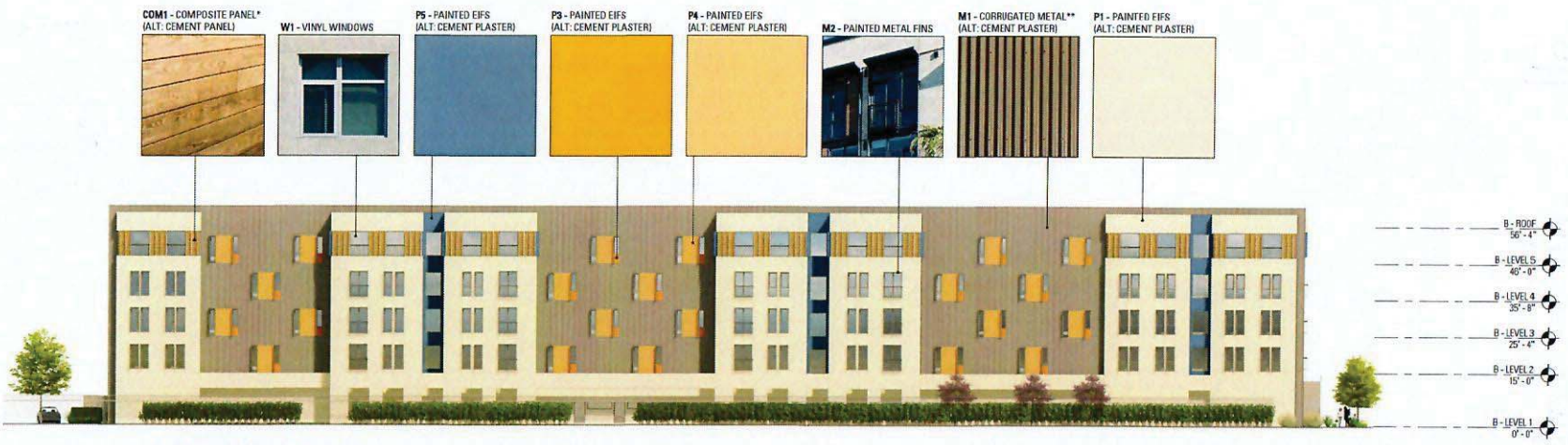
1 EAST ELEVATION - BLDG B A401A 1/16" = 1'-0"
