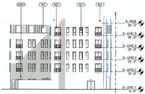
2 SOUTH ELEVATION - BLDG B A302 1/16" = 1'-0"
