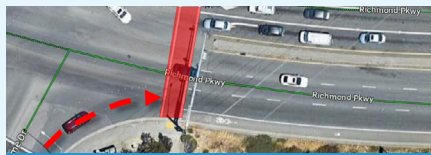
Corner sight distance issues
