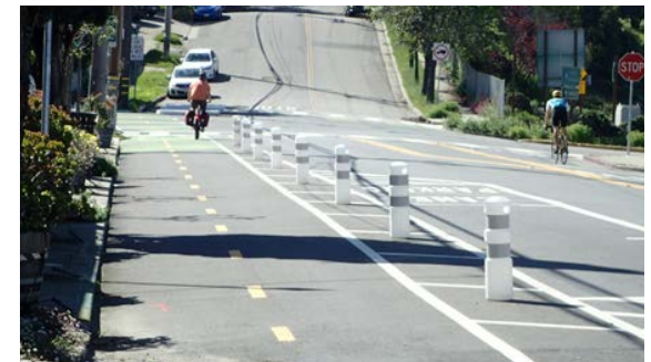
Existing cycle track on Tewksbury Avenue to be extended.
